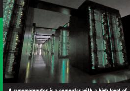
A supercomputer is a computer with a high level of performance as compared to a general-purpose computer. The performance of a supercomputer is commonly measured in floating-point operations per second (FLOPS) instead of million instructions per second (MIPS)
